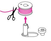
9. Cut the thread and then remove the bobbin.
