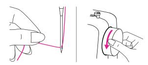
Hold the upper thread with your left hand. Turn the handwheel towards you (counterclockwise) to lower the needle down below the needle plate then raise it to bring the bobbin thread up.
