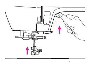
When sewing multi-layers or thick fabrics, the presser foot can be further raised up manually to allow enough space for your sewing work.
