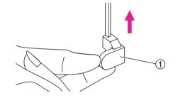
Raise the presser foot and cut the thread. To sew over the same buttonhole, raise the presser foot (it will return to its original position).
