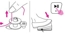
6. Push the bobbin to the right. When the bobbin winder spindle is pushed to the right, the screen will show "SP".
