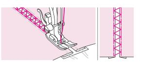
Align the center of the presser foot with the center of the two pieces of fabric and begin sewina.
