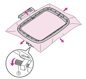
Place the inner hoop on the fabric and press firmly until them are securely fit to outer hoop perfectly. If the inner hoop cannot fit properly, loosen the outer hoop's fastening screw and adjust until fitted.
