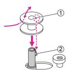
Place the thread end through one of 5. the inner holes as illustrated and place the empty bobbin on the bobbin winder spindle. Then align the notch with bobbin winder spindle spring.
