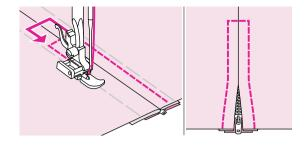
Stitching around the zipper. Remove the basting and press.
