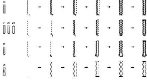
\* Buttonholes are sewn from the front of the presser foot to the back, as shown.
