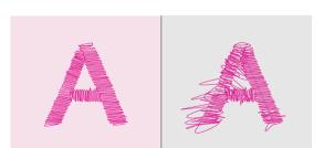
When the upper thread has slack, the thread tension is too loose for embroidering. To increase the tension, press the "+" button.
