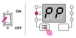
Turn on the power, and check if the screen shows "PP" and the second light is on. If it is not, please long press the connection mode switch button to switch the light.
