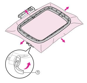
Place the inner hoop on the fabric and press firmly until them are securely fit to outer hoop perfectly, pull the fabric from the four sides marked with the arrows so that the fabric is stretched drum-tight in the hoop, and then press the inner hoop downwards so that it sinks into the outer hoop a little and close the quick release device.
