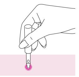
Make a hole at the center using an eyelet punch.
