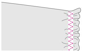
While pulling the fabric behind the presser foot with your left hand, pull the fabric at the pin nearest the front of the presser foot with your right hand.
