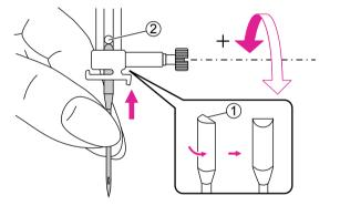
When inserting a new needle, keep the flat side of the shaft to the back.
