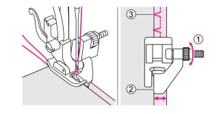
Place the fabric under the foot. Turn the handwheel forwards until the needle swings fully to the left. It should just pierce the fold of the fabric. If it does not, adjust the stitch width accordingly. Adjust the guide by turning the knob so that the guide just rests against the fold.
