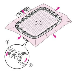
Place the inner hoop on the fabric and press firmly until them are securely fit to outer hoop perfectly. If the inner hoop cannot fit properly, loosen the outer hoop's fastening screw and adjust until fitted.
