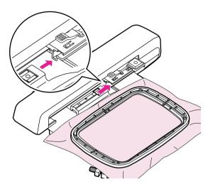
The embroidery hoop has two built-in sizes which are 120x80mm and 50x70mm, respectively. Select the corresponding size according to the image design.
