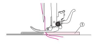
You also can place another piece of fabric with the same thickness at the back of the seam. Or support the presser foot while feeding by hand and sewing toward the folded side.
