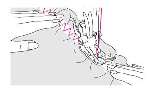
Sew the elastic tape to the fabric while stretching the tape so that it is the same length as the fabric.
